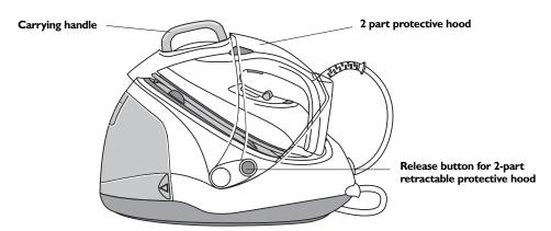
Your steam generator is equipped with an automatic "Security Auto-stop" function which cuts off the heating of the appliance when the flaps are closed over the iron. The control panel lights go out and the on indicator remains lit, showing that the appliance is connected but not heating.
